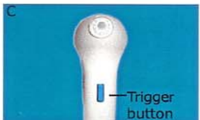
Press Trigger Button once to began calibration, again to end.
